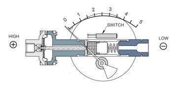
Model PR 20 consists of a convoluted diaphragm to sense the pressure difference. It can withstand maximum operating pressure up to 100 bar for all ranges. If pressure exceeds the rated maximum pressure, "O" rings & diaphragm inside the pressure chamber, will be damaged. If maximum operating pressure is within the allowable limit of 100 bar, but the differential pressure exceeds instrument range, there will be no damage to the instrument. Pointer will only go the extreme right end of the scale.
